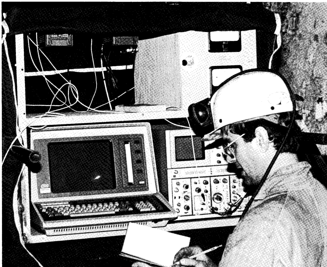
FIGURE 3. - Radar control console of GPR used during underground testing.
