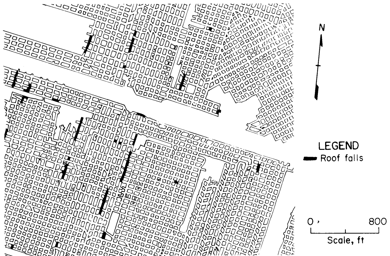
Figure 11.—Partial mine map from western Pennsylvania, showing preferential orientation of roof falls.
