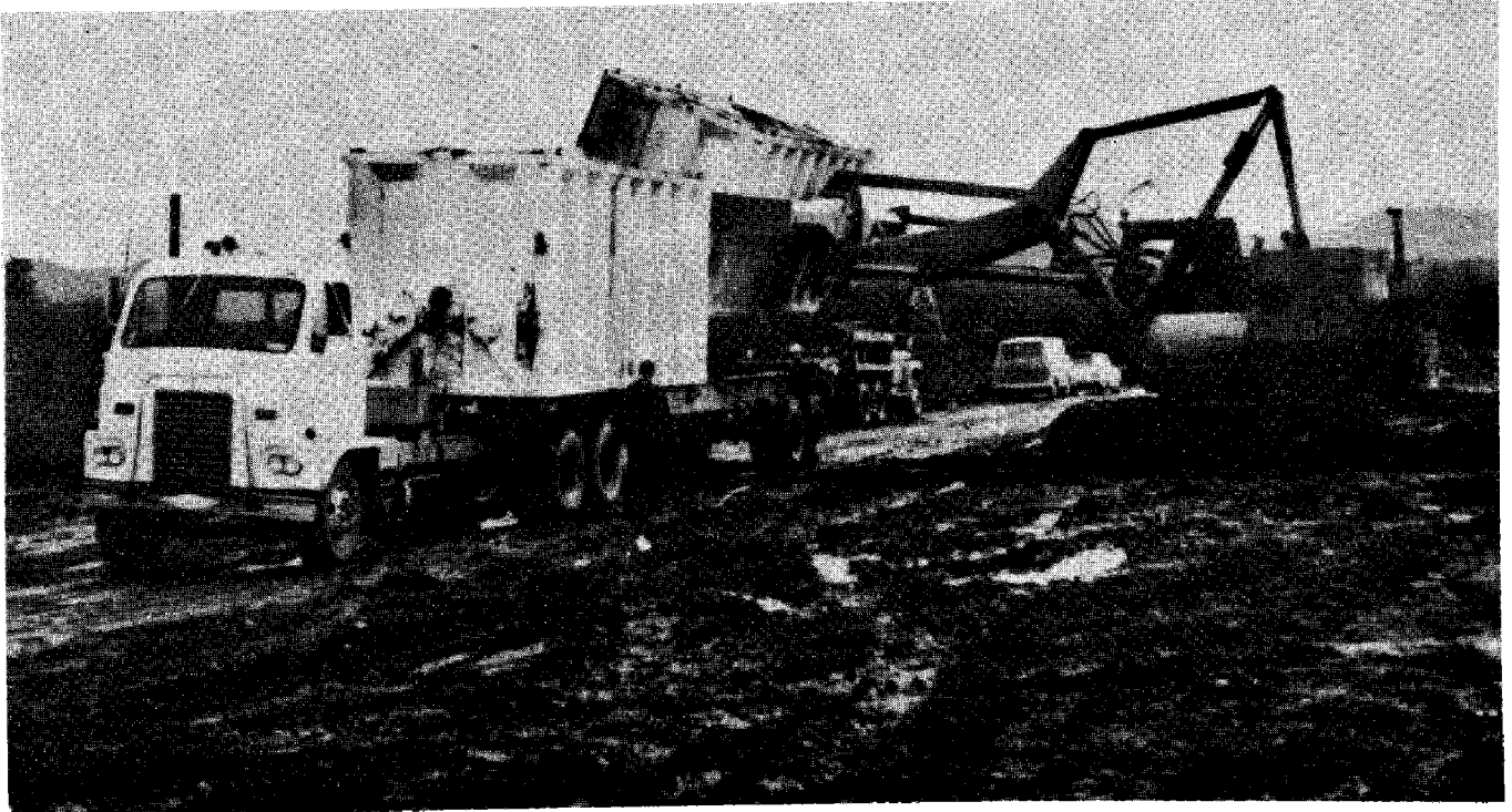
Special trailer hauls two refuse containers from transfer station to landfill site. Modified power shovel removes containers from trailer.
