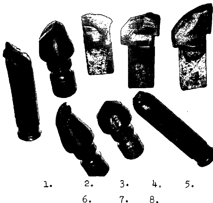
Figure D-5. Examples of Wear Patterns of Continuous Miner Bits from Company C, Mines 5, 6, 7, and 8
