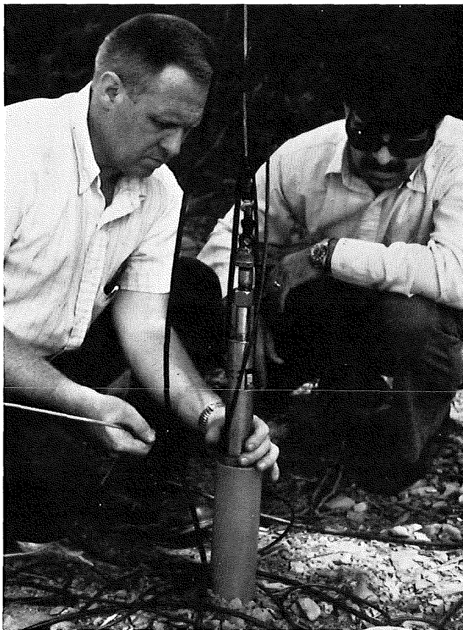
Figure 31 - Inserting Probe into Borehole Casing
