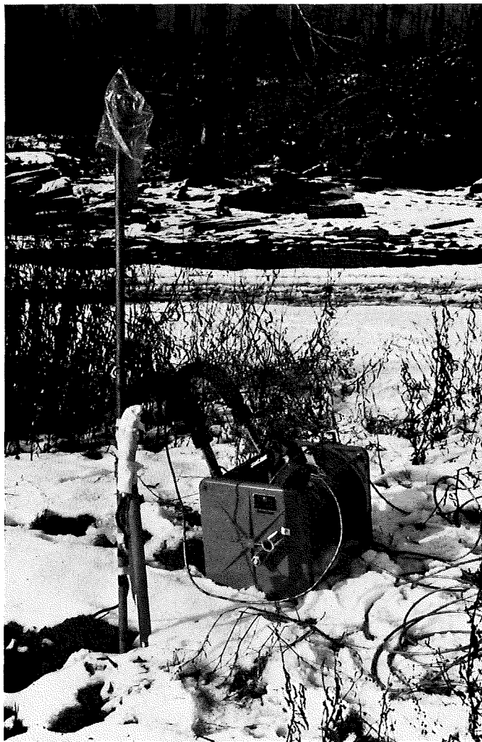
Figure 25 - Shallow Burial Geophone Site in Winter (Cable reel and line junction box shown, preamplifier is in insulated package taped to mounting post)
