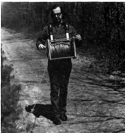
(A) Running Out Transducer Cable
