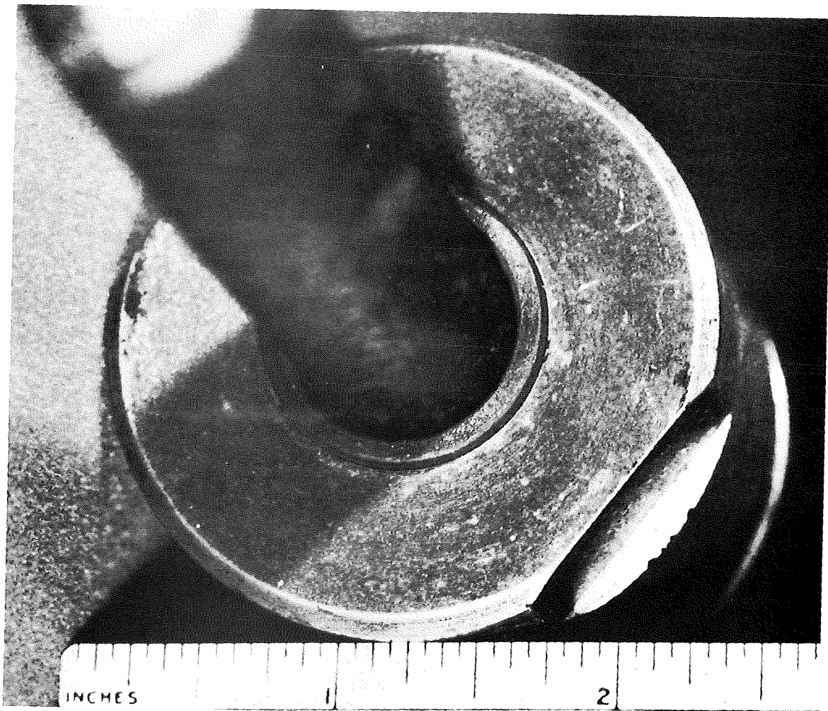
Figure 5-3. Grommet Tight Around Cable After Tightening Compression Nut
