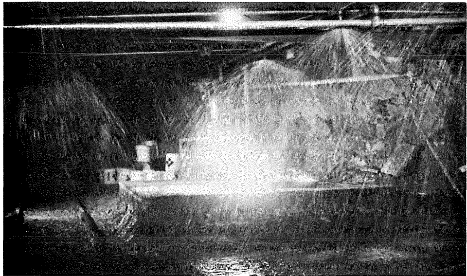
Figure 70 - Fire Test No. 1 - Foam Discharge (5 Seconds)
