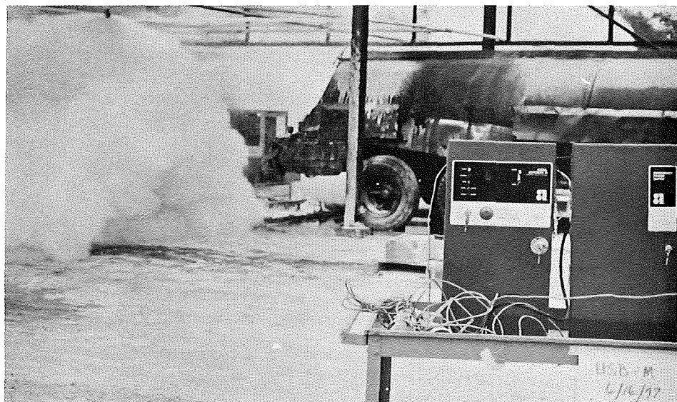
Figure 57 Fire Test No. 3 - Twin Agent System Discharge
