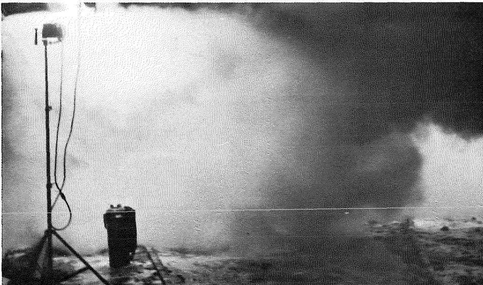
Figure 80 - Fire Test No. 2 Dry Chemical Discharge, Extinguishment (16 Seconds)
