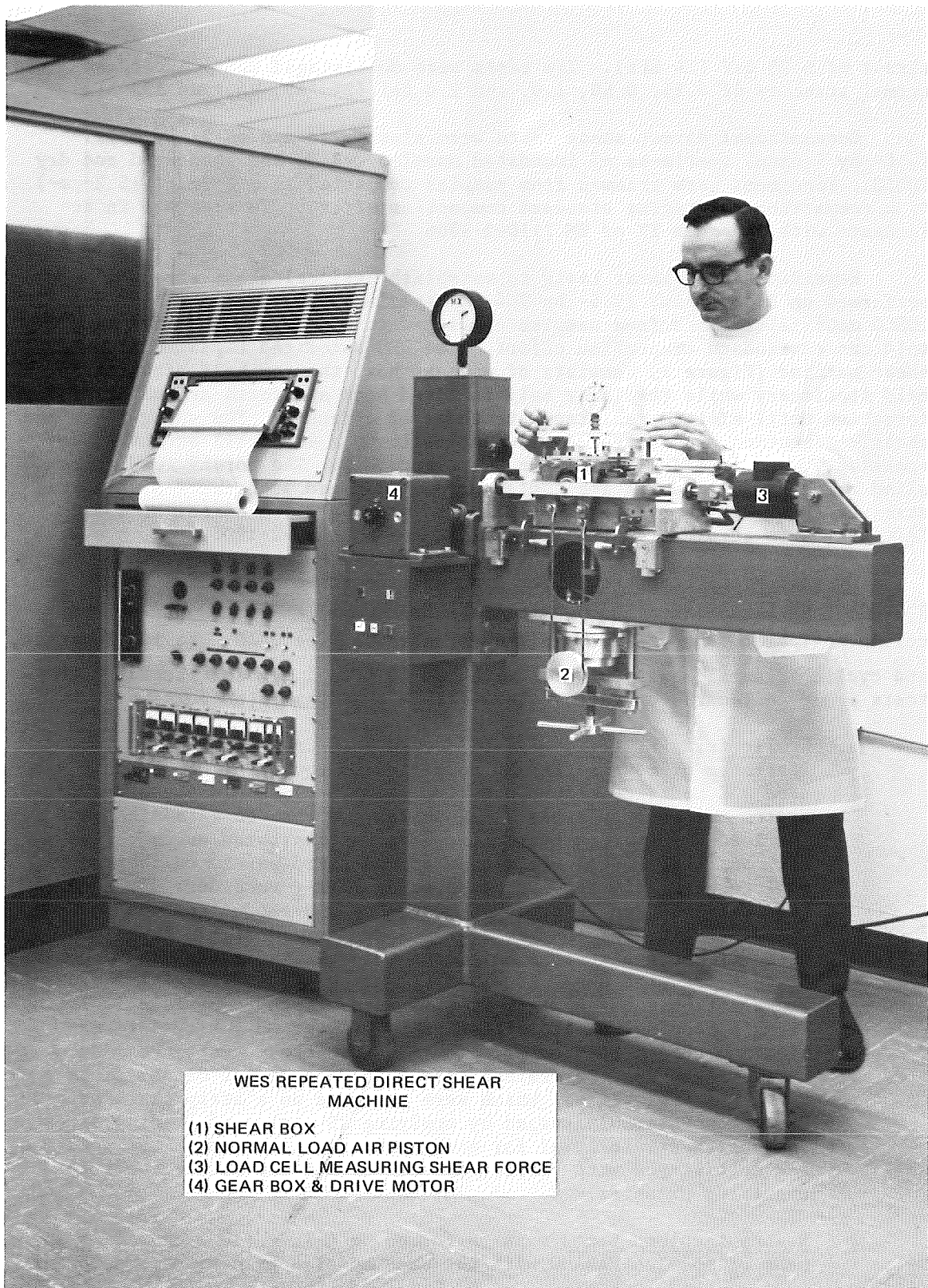
Figure 7. WES automated repeated direct shear machine
