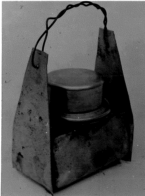
Figure 11 Radiator Capsule Assembled with Flux and Solder Ready for Processing
