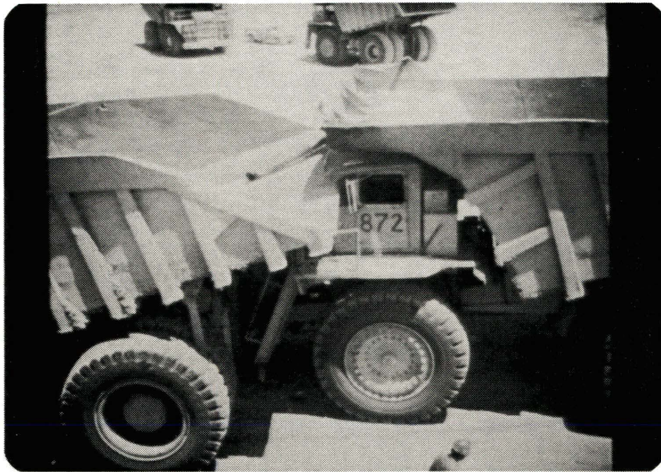
FIGURE 4-1. Haulage Truck Backing Into Parked Haulage Truck
