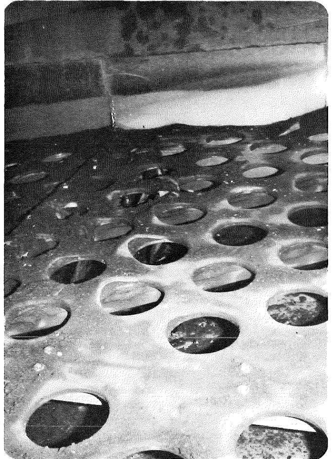
FIG. 23. SEPARATION OF TUFFGARD-80 DUROMETER LAYER FROM STEEL SCREEN AFTER 2 MONTHS OF USE.
