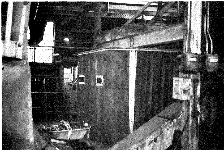
FIG. 51. CURTAINS INSTALLED AROUND MIDDLEING SHAKERS.
