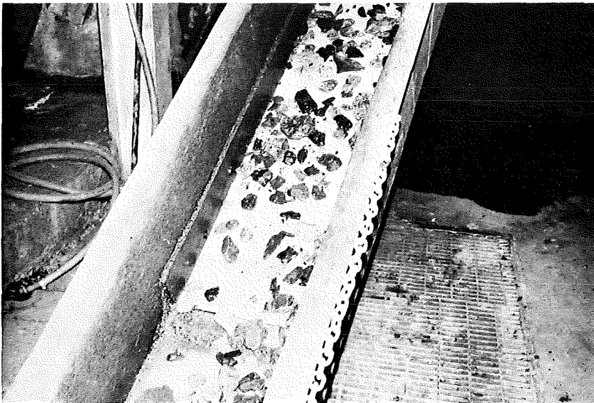
FIG. 45. MINALOY PLASTIC CHUTE LINER IN NO. 2 JIG REFUSE CHUTE.
