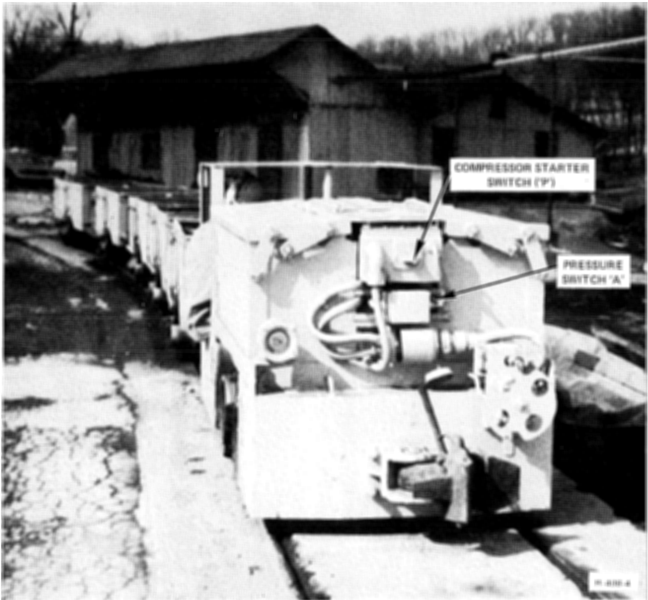
Figure 4-11 - Electric Locomotive - Battery Box End
