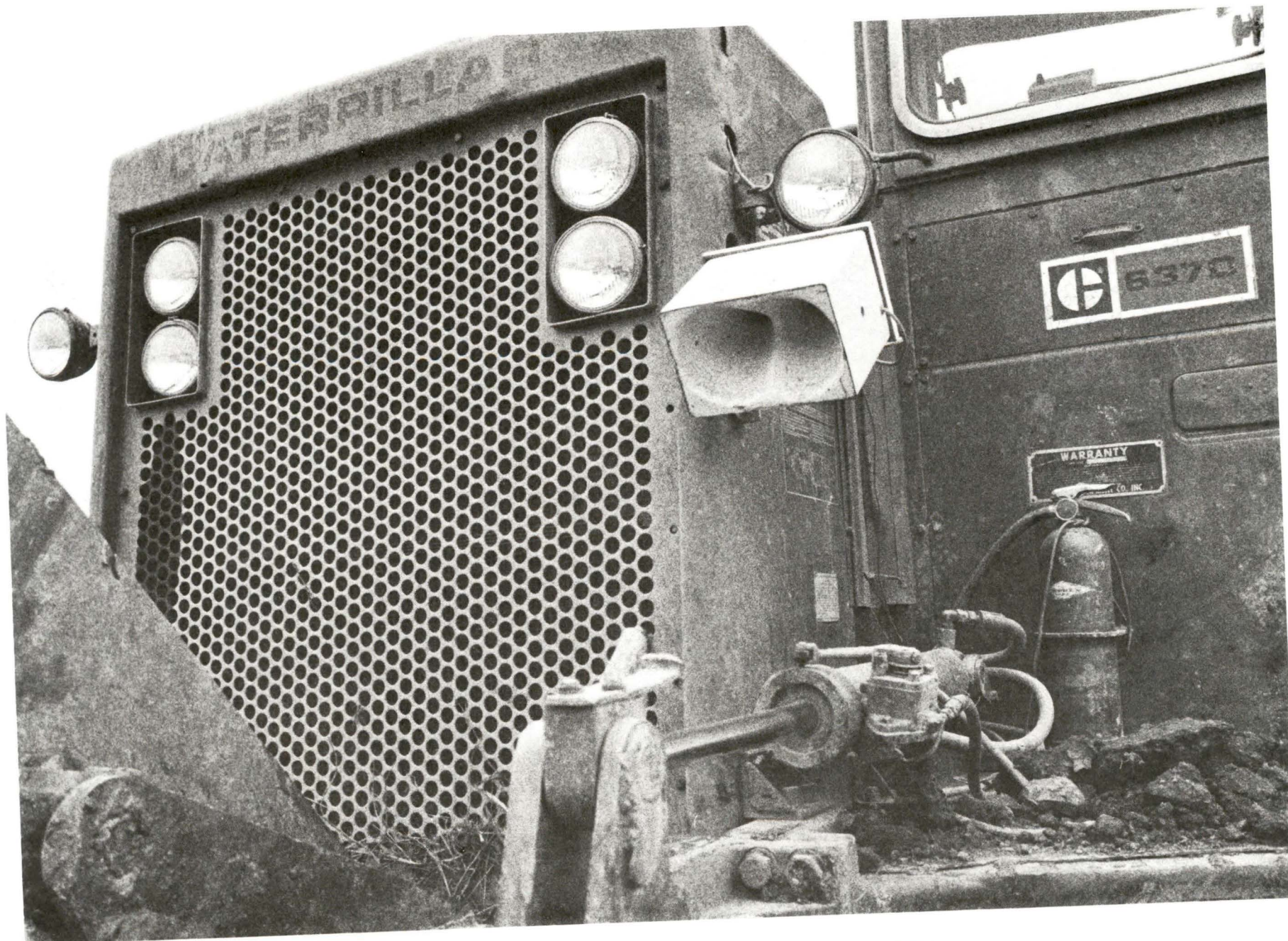
FIGURE 41. GROUND SPEED SENSOR MOUNTING FOR WORKING MINE FIELD TESTS
