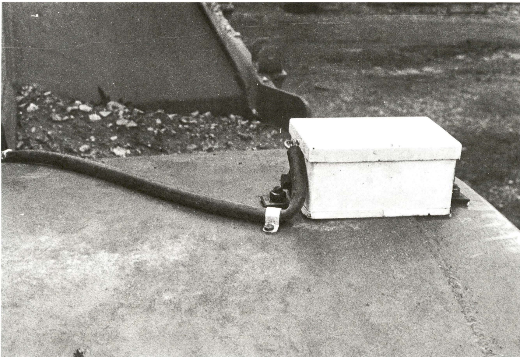
FIGURE 25. CATERPILLAR 637D LEFT FRONT WHEEL SPEED SENSOR INSTALLATION
