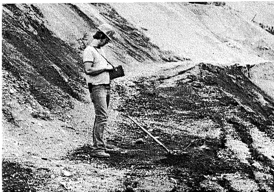
Gas sample being taken above vapor chimneys (station 4 + 00-3).
