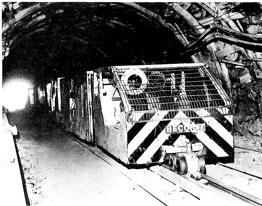
FIGURE 28A. ROAD RAILER DIESEL LOCOMOTIVE (PHOTO COURTESY BECORIT (GB) LIMITED & NCB SOUTH DURHAM AREA)
