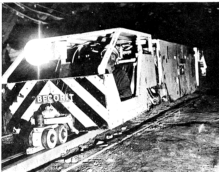
FIGURE 28B. ROAD RAILER DIESEL LOCOMOTIVE (PHOTO COURTESY BECORIT (GB) LIMITED & NCB SOUTH DURHAM AREA)
