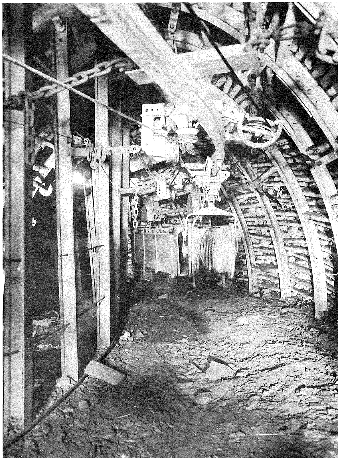
FIGURE 33. SCHARF MONORAIL TRAVELING IN LIMITED ROADWAY SPACE. NOTE CHAINS GIVING HORIZONTAL STABILIZATION TO CURVED TRACK SECTION. (PHOTO COURTESY MASCHINENFABRIK SCHARF GMBH.)
