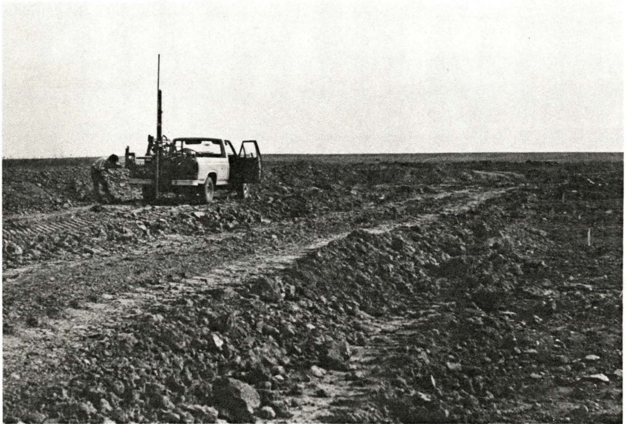
FIGURE 42. Sampling of Second Lift of Windrow Test Plot Following Scraper Soil Replacement
