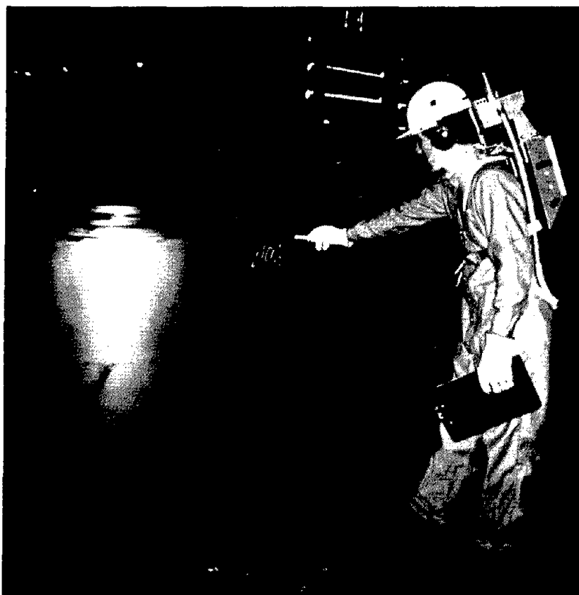
Figure 7. Illustration of a fully instrumented test subject carrying personal heat stress monitor
