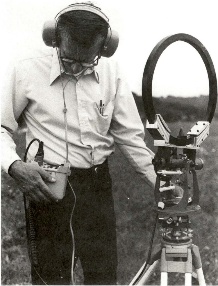
FIGURE 6. - Receiver coil mounted on transit.
