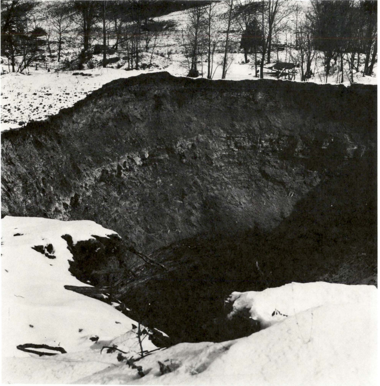
FIGURE 15. - Soil profile of weathered in situ rock at north end of Bautsch mine failure.
