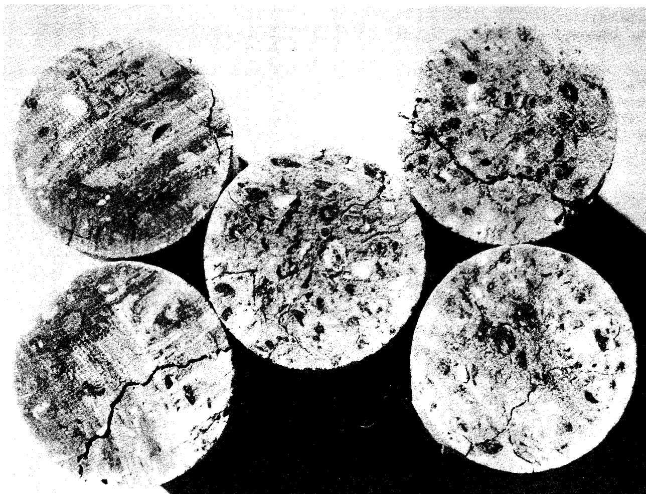
FIGURE 5. - Unmodified concrete cylinders after aging in humid conditions;
