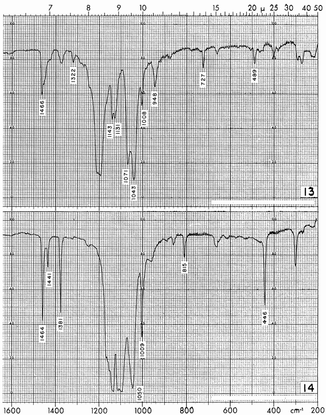
FIGURE 11. - Spectra of (13) zinc n-amyl xanthate and (14) potassium ethyl xanthate.-Continued
