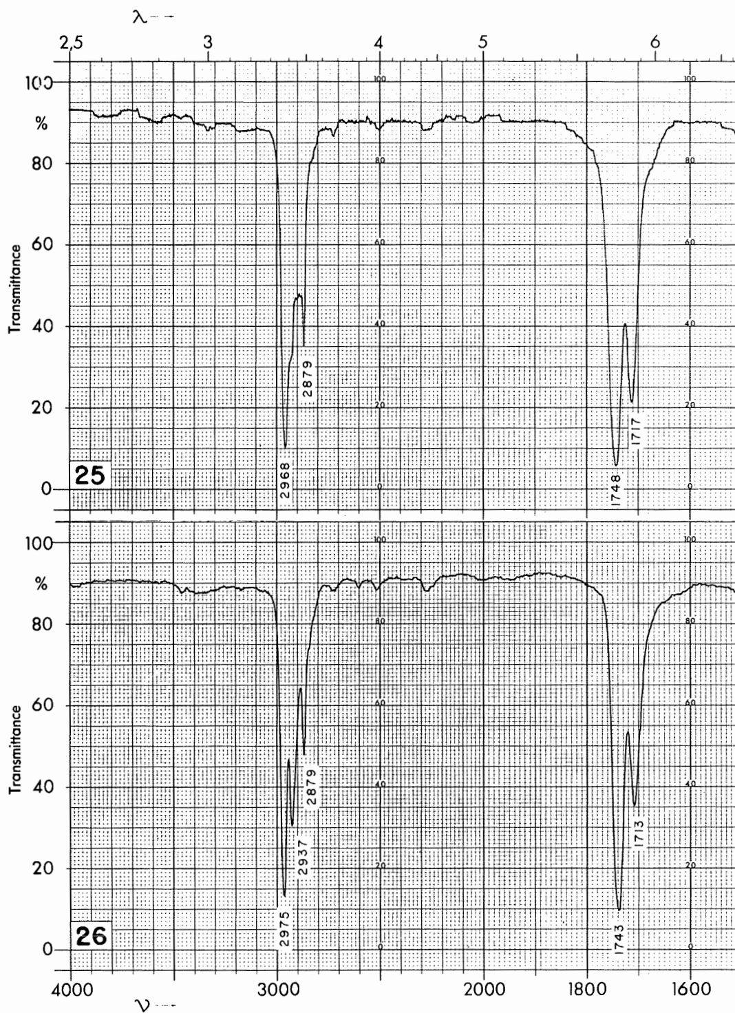
FIGURE 17. - Spectra of (25) di-isobutyl dixanthogen and (26) di-secondary-butyl dixanthogen.
