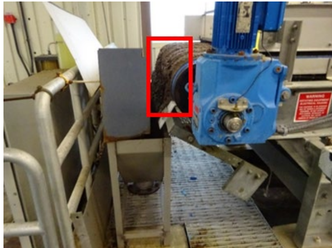
Figure B7. Solid sludge on conveyor belt to collect sample. Photo by NIOSH.
