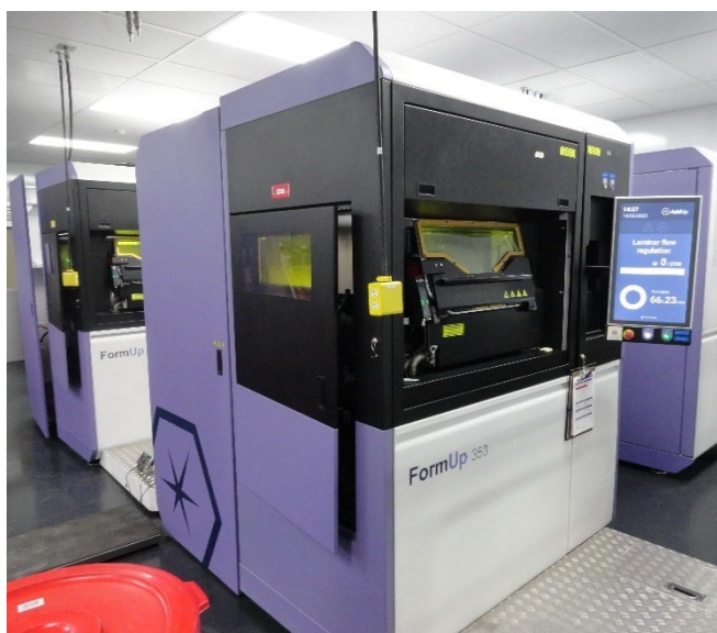
Figure A1. A powder bed fusion machine on standby. Photo by NIOSH.
