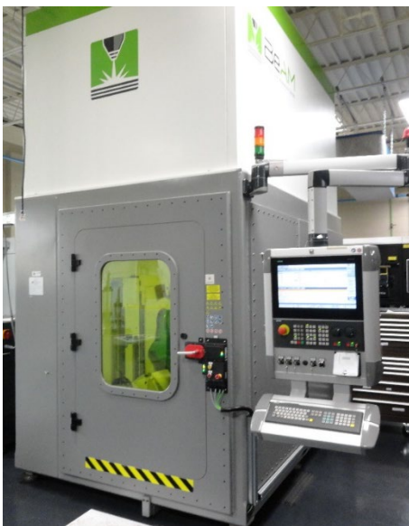
Figure A3. A directed energy deposition machine on standby. Photo by NIOSH.
