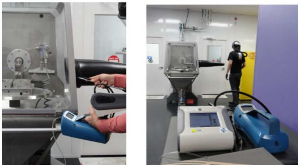
Figure B29. Sampler placement for the depowdering task: (a) near field monitors were held by a NIOSH staff person, (b) location of far field basket. Photos by NOISH.
