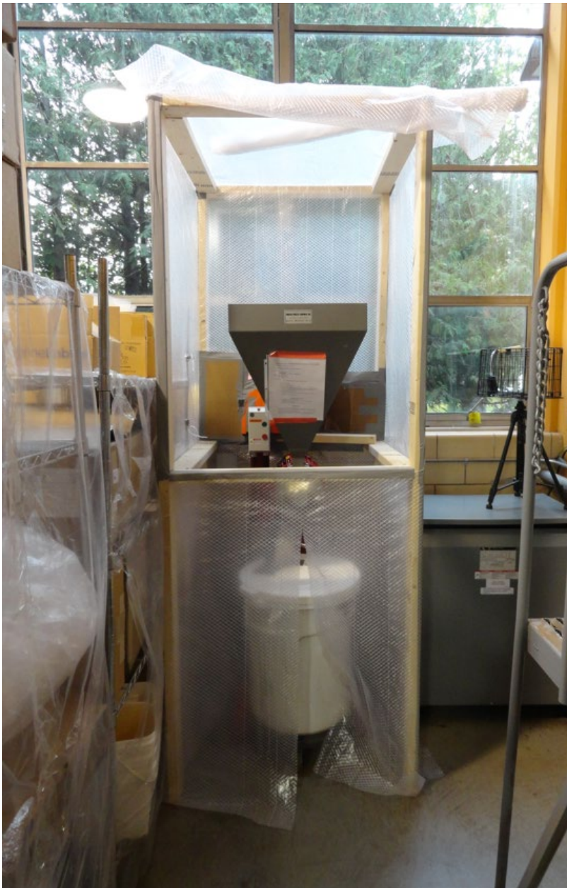
Figure B1. Ventilated enclosure installed at the large grinder with movable flap rolled up to allow access. Photo by NIOSH.
