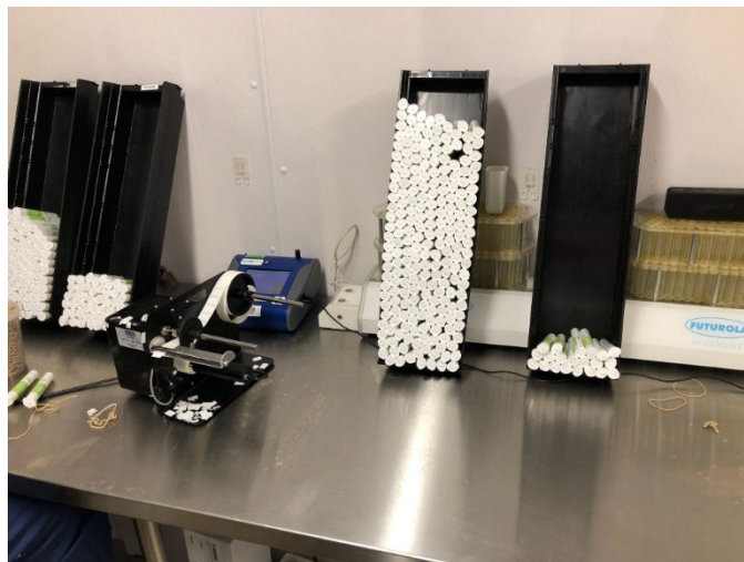
Figure A3. Pre-roll workstation showing the knock-out boxes, containers, and labeling equipment. A DustTrak® is shown in the background, which measures aerosols generated during the work tasks. Photo by NIOSH.
