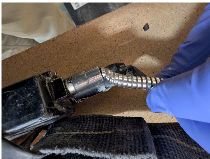
Photo 2 (top) & 3 (bottom): Show damage to the high-pressure hose near the PASS device of the deceased firefighter's SCBA. (Courtesy of NIOSH)
