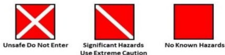
Diagram 2: IAAI/USFA high-risk building marking system (Courtesy of USFA)
