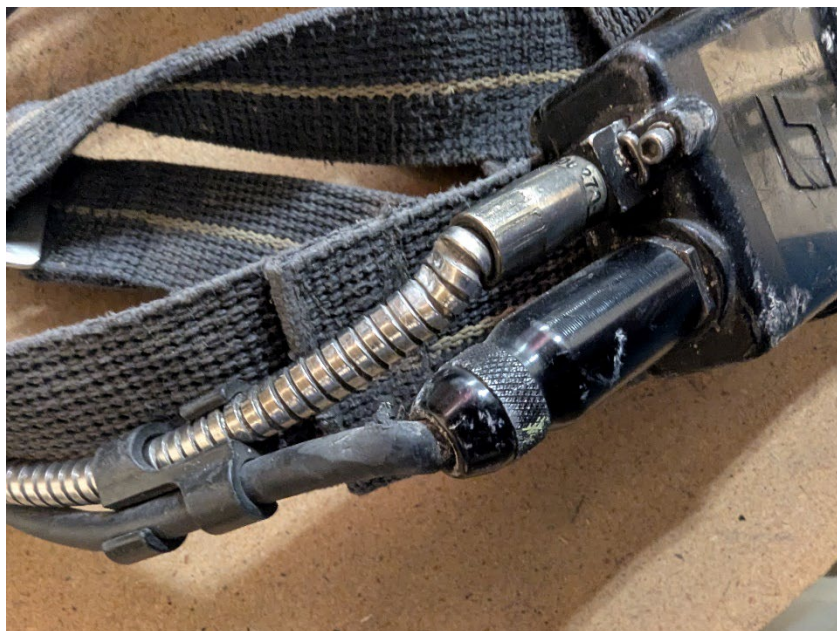
Photo 2 (top) & 3 (bottom): Show damage to the high-pressure hose near the PASS device of the deceased firefighter's SCBA. (Courtesy of NIOSH)
