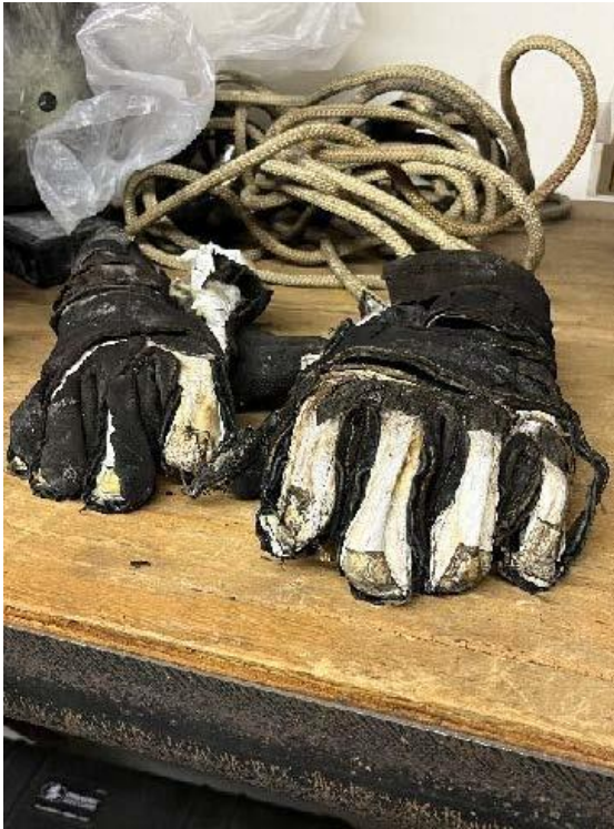
E31FF1's structural turnout gear (4a), gloves (4b), and portable radio showing extent of damage (4c). (Courtesy of NIOSH)
