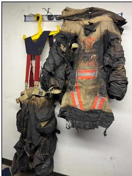
Photos 4a, b, and c: E31FF1's structural turnout gear (4a), gloves (4b), and portable radio showing extent of damage (4c). (Courtesy of NIOSH)
