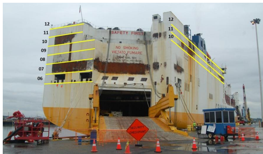
View of the vessel from the rear/stern with the deck levels noted. The rear/stern vehicle ramp is shown, which was used by all personnel during the incident to access deck 3. (Courtesy of NIOSH)
