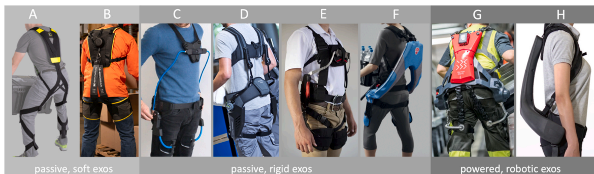
Fig. 1. Examples of commercial back exos. Passive, soft exos (i.e., elastic exosuits made primarily from soft materials): A) Kinetic Edge Flex Lift, B) HeroWear Apex. Passive rigid exos (i.e., elastic exoskeletons made primarily from rigid components): C) Laevo, D) Ottobock Paexo Back, E) SuitX BackX, F) Innophys Muscle Suit Every. Powered robotic exos (i.e., using motors to assist): G) German Bionic Cray X, H) Atoun Model Y. Regardless of differences in componentry (rigid vs. soft) or actuation (passive vs. powered), each of these exos assists biomechanically by generating an extension moment (torque) about the lumbar spine during lifting, which reduces musculoskeletal loading on the user's low back.
