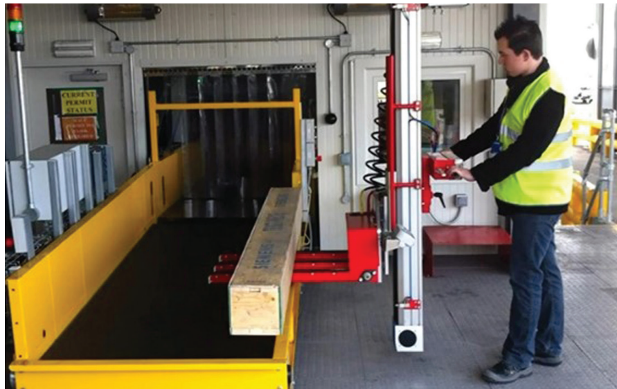
An example of an overhead fork design lift.
