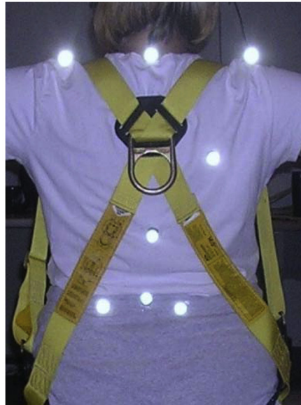
Fig. 1. Marker locations from the Plug-In Gait marker configuration. a) Anterior view: manubrium, xyphoid process, bilateral ASIS. b) Posterior view: C7, T10, L4, bilateral PSIS. Bilateral acromion processes are apparent in both views. Other markers can be seen in the photographs that are part of the Plug-In Gait set but not used in determination of thorax and pelvic kinematics. The subject is wearing a harness which was connected to a gantry system to prevent a fall during trials of staircase locomotion, as presented in [18].
