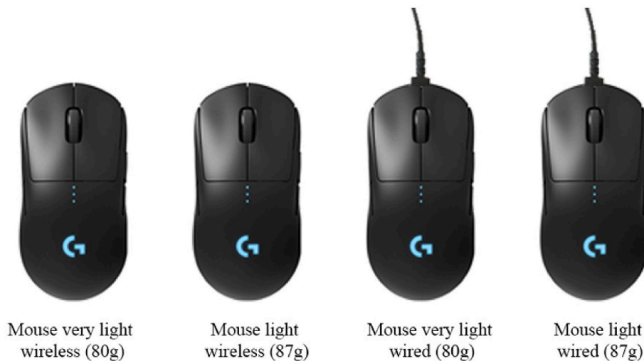
Fig. 3. Four experiment mice: very light wireless mouse (80g), light wireless mouse (87g), very light wired mouse (80g) and light wired mouse (87g), identical in appearance.
