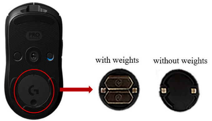
Fig. 4. The back of experiment mice. The rear cover was shown in two conditions: with 7-g weights (87g) and without weights (80g).
