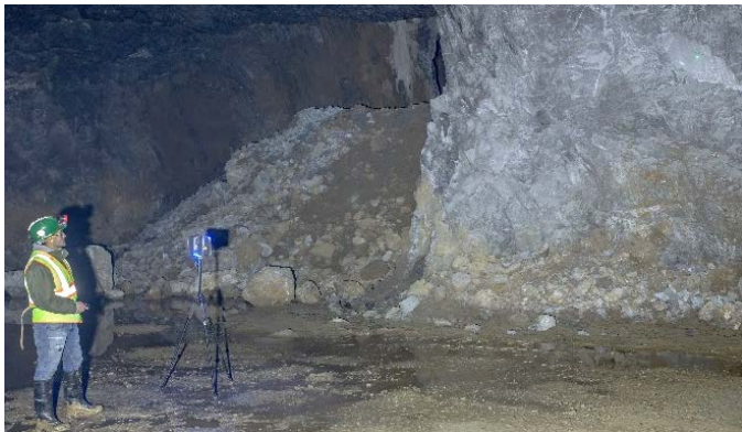
Figure 6. Laser scan of limestone mine pillar.
