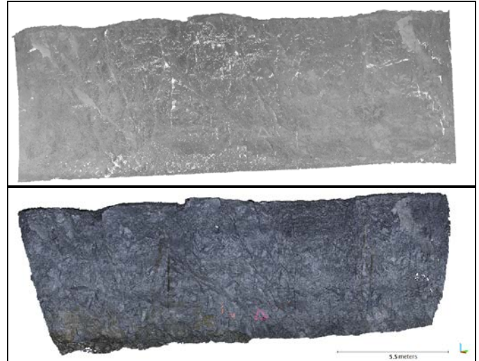
Figure 7. Point Clouds – Laser Scan (top) vs Photogrammetry (bottom) from CloudCompare.
