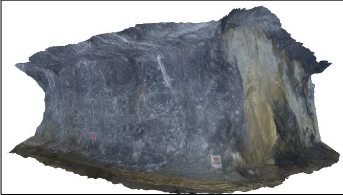
Figure 2. Three-dimensional rendering of subject pillar using photogrammetry.
