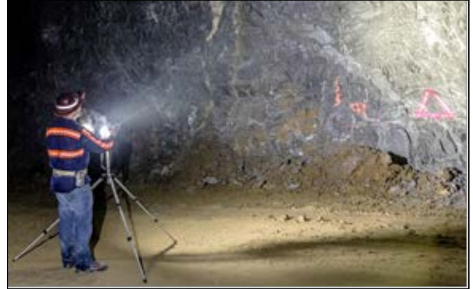
Figure 4. Photogrammetry survey of mine pillar.
