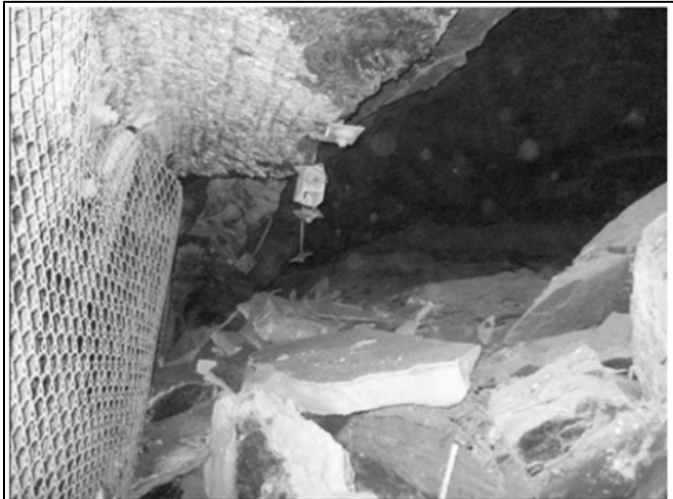
Figure 1. The edge of a longwall gob near the mining face at a western U.S. coal mine [10]. Notice how the size of the rock rubble gets smaller looking further back into the gob.
