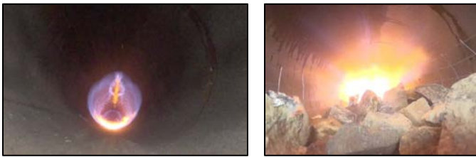
Figure 5. Left - The stoichiometric methane flame in the initial run up inside the empty 71cm diameter reactor. Right - The flame accelerates dramatically when the rocks are encountered. This image shows the flame over the first part of the rock insert in the 71cm reactor. Tests performed at a mean of 76kPa and 294K.
