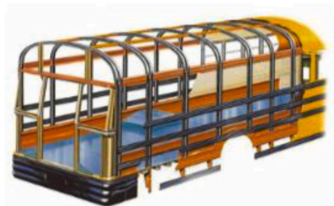
Fig. 2. School bus roof structure (courtesy of Blue Bird Corporation). (For interpretation of the references to colour in this figure legend, the reader is referred to the Web version of this article.)
