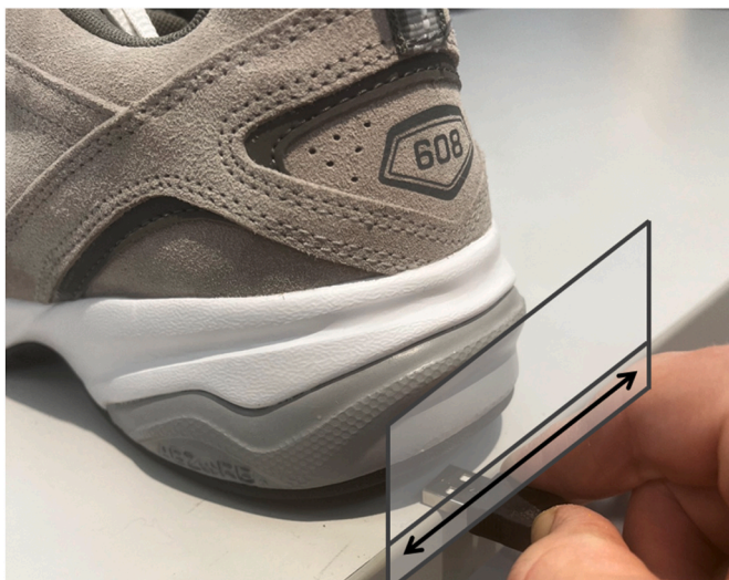
Fig. 1. The test used to assess whether shoes contained a bevel. The back of the heel and the back of the USB latches (rectangular holes) were aligned with the side of a table. If there was enough space to accommodate the portion of the USB port in front of the latches, the shoe was considered to be beveled.
