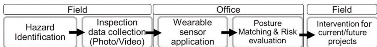
Fig. 1. Concept of the inertial sensor-based posture-matching method.
