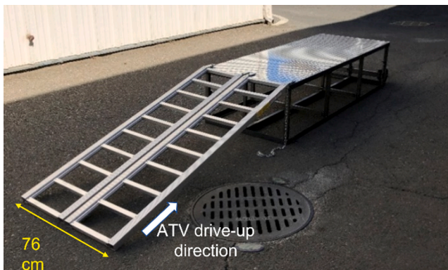
Fig. 13. Ramp for ATV rollover tests.
