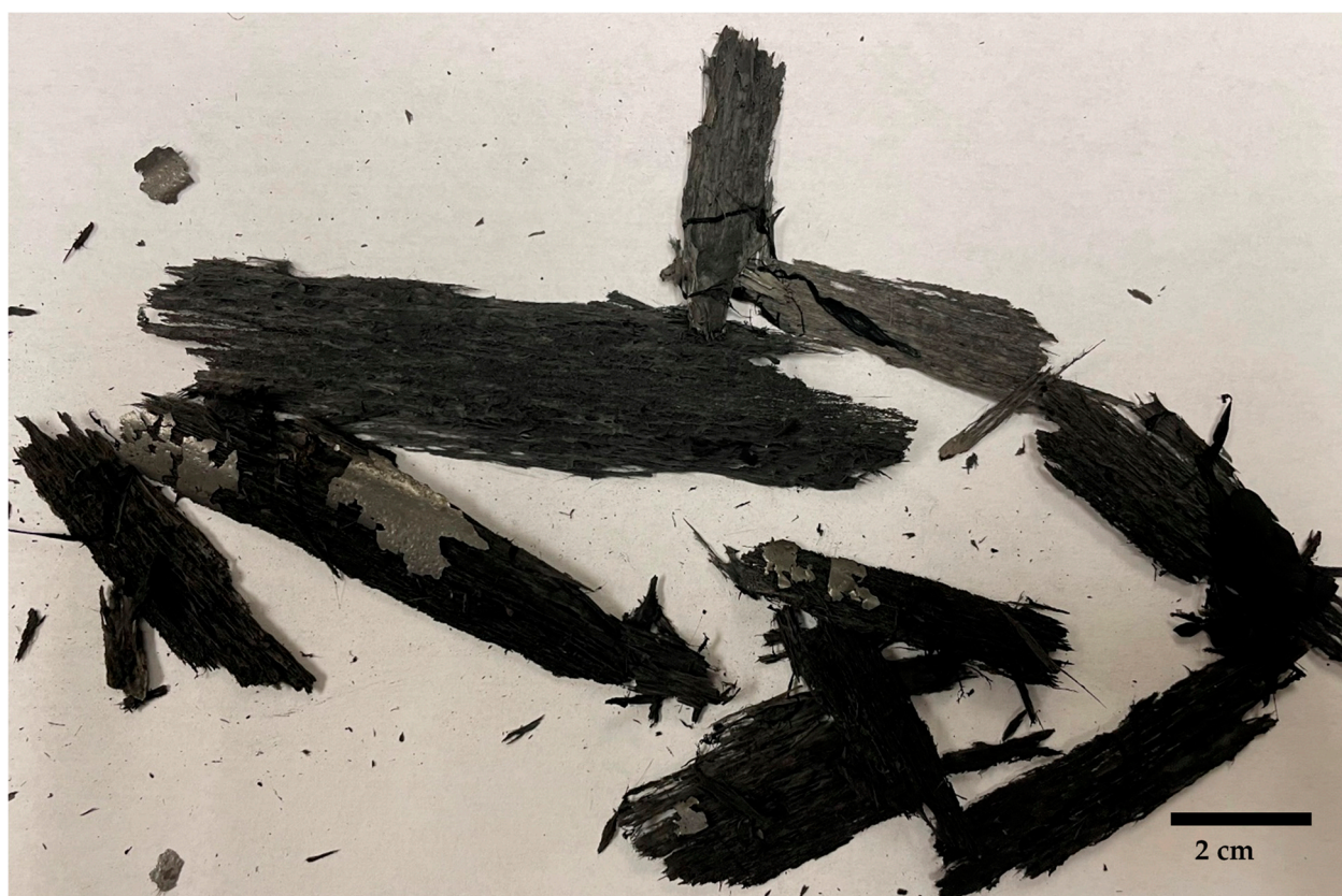
Figure 10. Deposits from the reactor tube after experiment.
