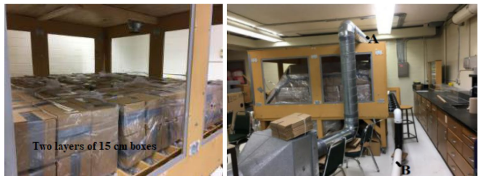
Fig. 18 Two layers of 15 cm boxes used in case 2 (left); overview of the cave model and fan setup (right)
