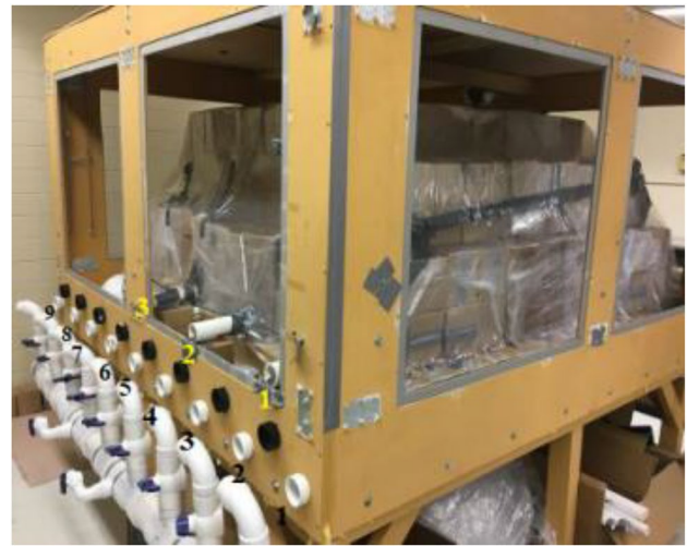
Fig. 2 Nine extraction and three undercut drift inlets
