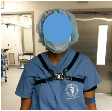
Figure 1. Surgeon wearing the wireless sensors used to record motion (sensors with black straps) and muscle activity (not seen, on the posterior side of the surgeon) during surgery.
