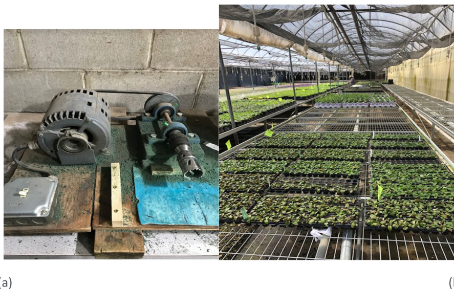
Fig. 3. Problem areas identified included (a) unguarded equipment used for pot hole drilling and (b) narrow walkways for plant transport.
