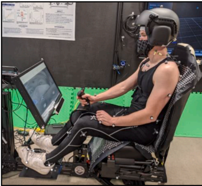
Fig. 1. Picture of H-60 cockpit setup.
