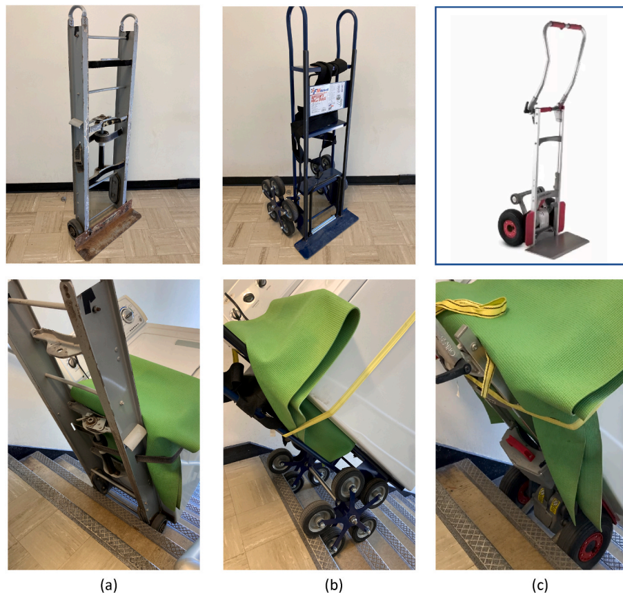
Fig. 1. The three hand truck designs used in the study included a “conventional” (a) used for appliance delivery, the multi-wheel design (b), and the powered stair ascending/descending hand truck (c).
