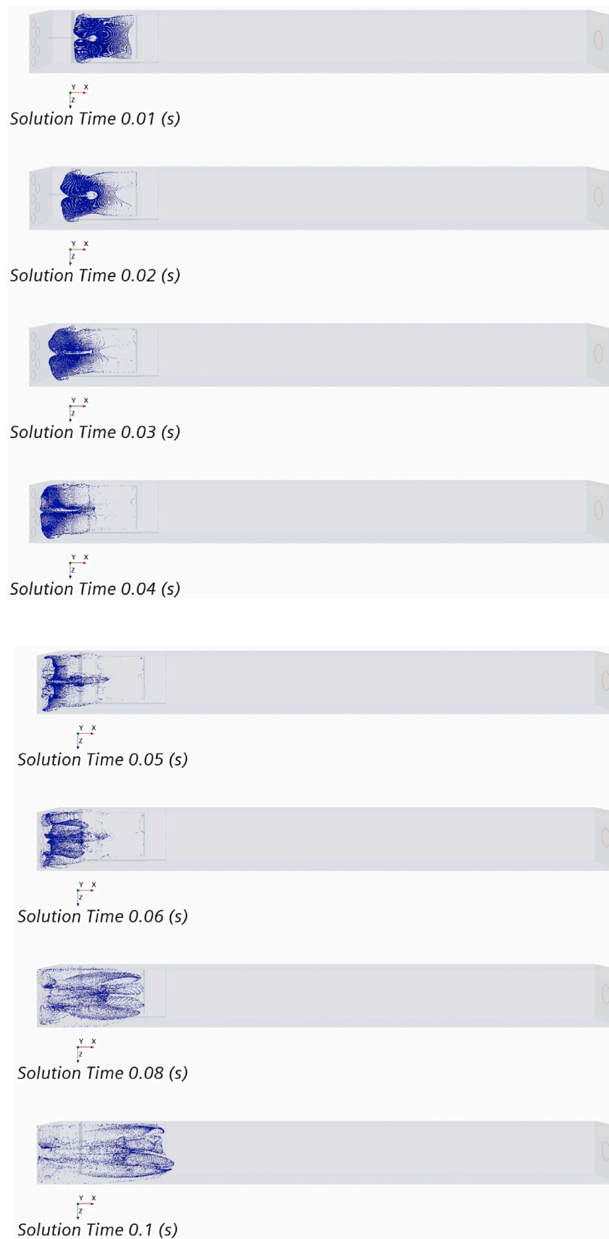
Fig. 4. Top view of the dispersing of 1\ \mu\text{m} particles. Particle locations (throughout the domain) in dark blue. Times: 0.01, 0.02, 0.03, 0.04, 0.05, 0.06, 0.08, 0.1, 0.25, 0.5, 0.75, 1 s. (For interpretation of the references to color in this figure legend, the reader is referred to the Web version of this article.)
