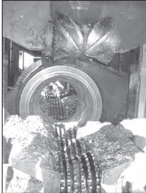
An incident with a debarker in 2008 involved maintenance on a debarker machine. The worker was crushed under the heavy press roll (at top) when hydraulic pressure was released.
