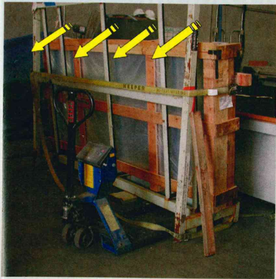
"L" rack with manual pallet jack positioned in open space beside forklift pocket. In this incident, two pallet jacks were used: one on each side. Arrows indicate direction the "L" rack toppled.
