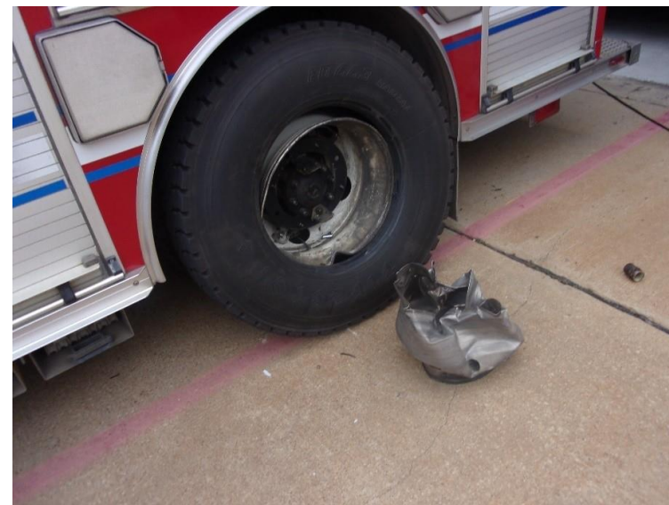
Apparatus tire that came off the wheel rim while being refilled with air. (Courtesy of the fire department)
