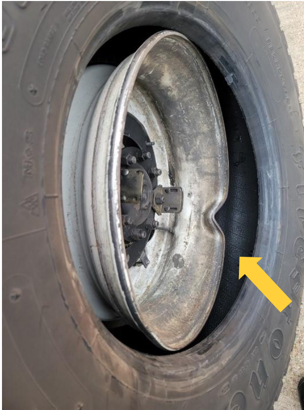
Rim deformation passenger side rear of Engine 4. (Courtesy of the fire department)
